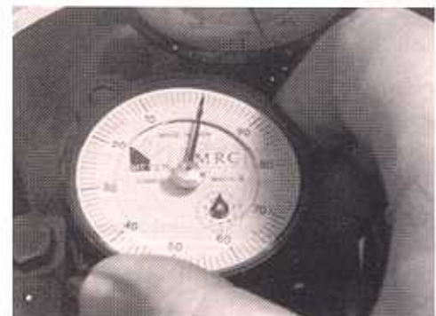
(Fig. S-3) Loosen the thumb screw and adjust the indicator to double zero.
