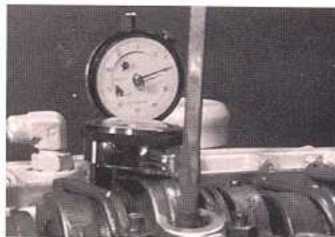
(Fig. T-2) Adjust timing using a 19mm wrench and a flat head type screwdriver. Turn screw until the indicator matches the calculated reading.
